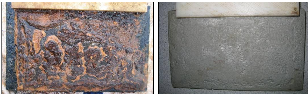
Figure 2. Uncoated Test Coupon Before and After Cleaning
